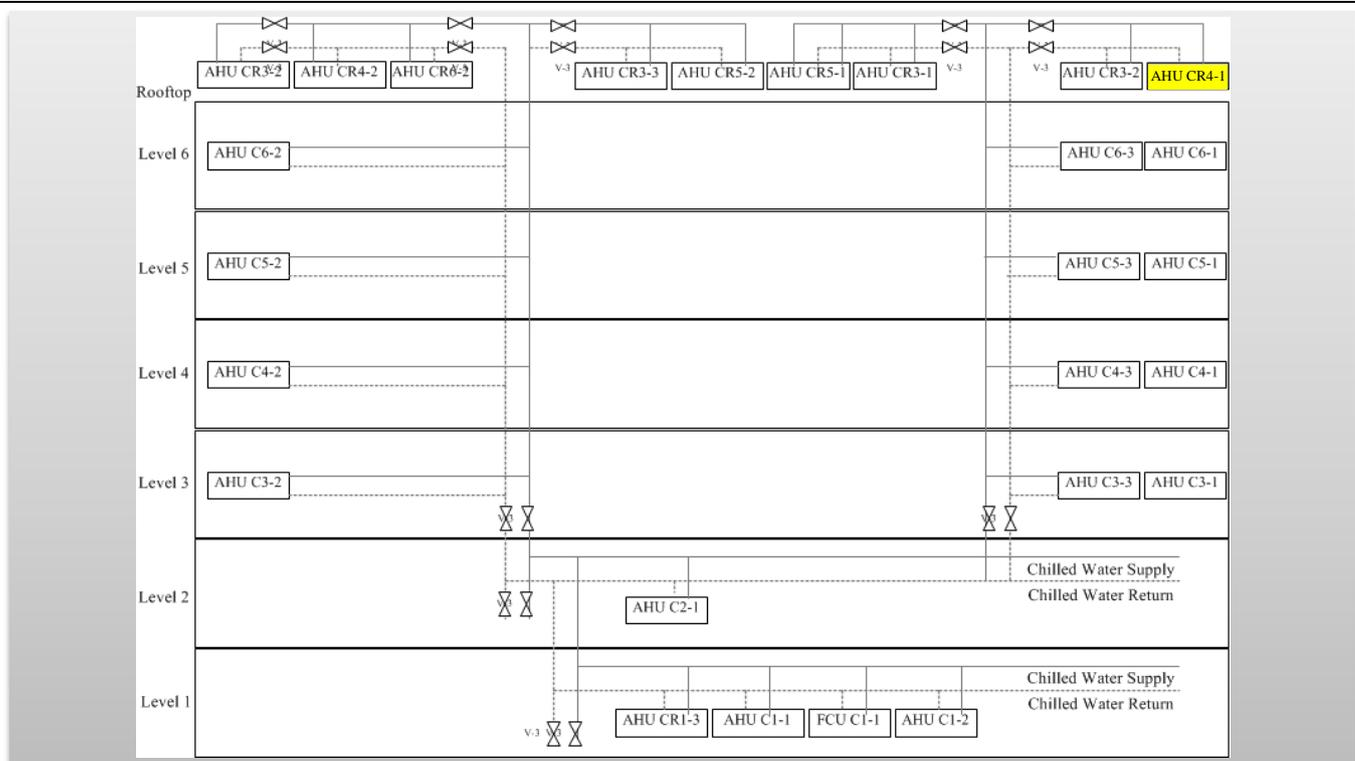
Figure 2: Air handling unit (AHU) schematic of the Chemistry Block at SPMS NTU with the highlighted AHU CR4-1 used for testing
