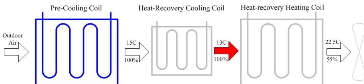
Figure 3: Control description of the AHU
