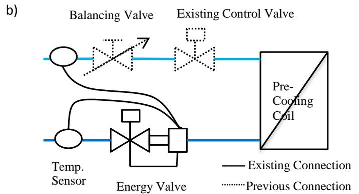
*Figure 4: a) The Belimo Energy Valve™; b) Installation schematic of the pre-cooling coil*
